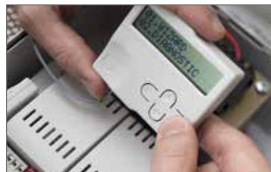
DYL handheld programmer with display for easy programming
